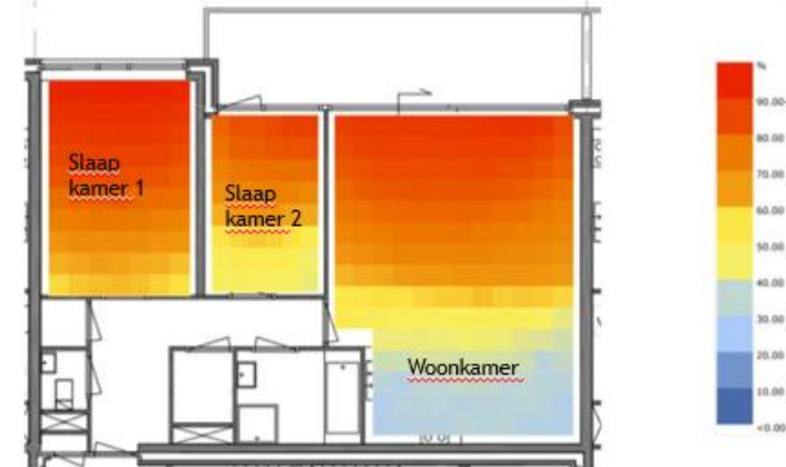
Figure 26 b) — Example showing south orientation with external shading with an LTA of 30 % with the percentage of the time that the illuminance is higher than 145 lx
