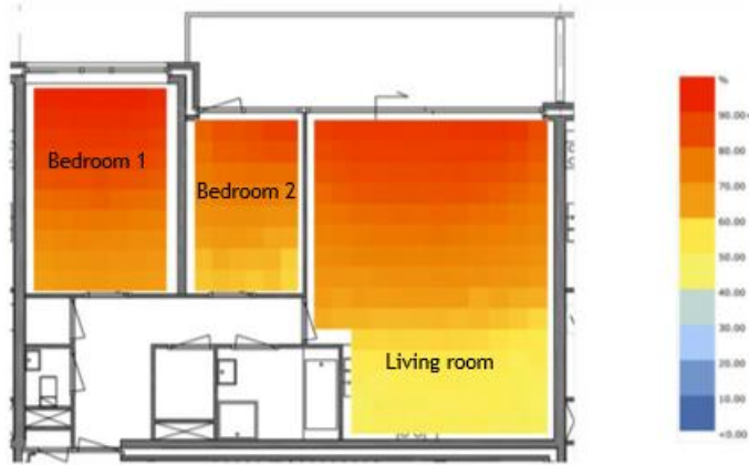
Figure 26 a) — Example with south orientation without shading with the percentage of time the illuminance is higher than 145 lx
